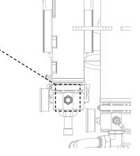
Figure 17. Removing and replacing the heating tank element. The heating system should be drained, cleaned and flushed annually. See **SECTION 4.3**.
