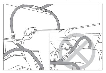
Figure 6. Typical coolant discharge ports installed on a turbocharged locomotive engine (above) and supercharged engine at Y-pipe (below). To distribute heat evenly, the return line is split into two discharge ports. Each port is installed at a welded 45° fitting, angled to ensure majority of heated coolant is transferred directly to engine block. Note incorrectly oriented fitting (inset). This fitting should be angled in the opposite direction to allow flow toward the engine.
