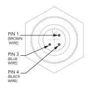
Figure 13. RTD pins 1, 3 and 4. The resistance between pin 1 and pin 3 should measure between 80 and 120 ohms. There should be continuity between pin 1 and pin 4.
