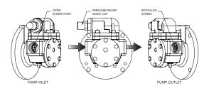
Figure 11. DLV oil pump assembly. Note that the pressure relief valve cap must always point toward the inlet side of pump. Screw is installed on outlet side of pump.
