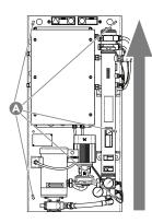
Figure 7. DLV 0.438 inch (11.13 mm) diameter mounting holes × 6 (A). Mount unit in orientation shown. Do not mount at an angle or in any other orientation.
