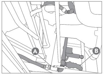
Figure 5. Coolant suction port installed at main locomotive engine drain. Note suction port (A) has been installed at the same level as the drain (B), ensuring DLV pump will draw water from the cooling system's lowest point.
