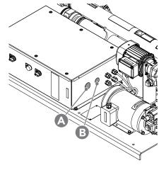
Figure 8. Underside of DLV control box, showing 1.25 " NPT main power entrance (A) and 0.5 " NPT customer interface wiring entrance (B).
