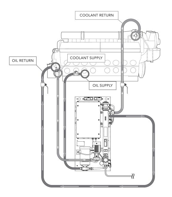
Figure 2. DLV operation overview, showing oil and coolant circulation. While the heating elements cycle on and off to maintain the preset temperature, the pumps circulate fluid continuously during operation.
