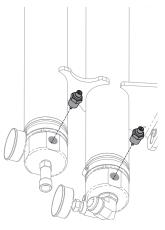
Figure 15. RTD plugs shown removed from DLV heating tanks.
