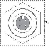
Figure 16. Proper RTD orientation. Note the notch centered at the top of the RTD connection.
