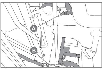
Figure 4. Typical oil discharge port **(A)** installed at locomotive engine lower P-pipe. Note coolant suction port **(B)** located at locomotive main engine drain.
