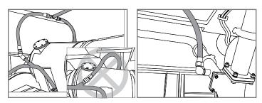
Figure 14. Typical coolant discharge ports installed on a turbocharged locomotive engine (left) and supercharged engine at Y-pipe (right). To distribute heat evenly, the return line is split into two discharge ports. Each port is installed at a welded 45° fitting, angled to ensure majority of heated coolant is transferred directly to engine block. Note incorrectly oriented fitting (inset). This fitting should be angled in the opposite direction to allow flow toward the engine.
