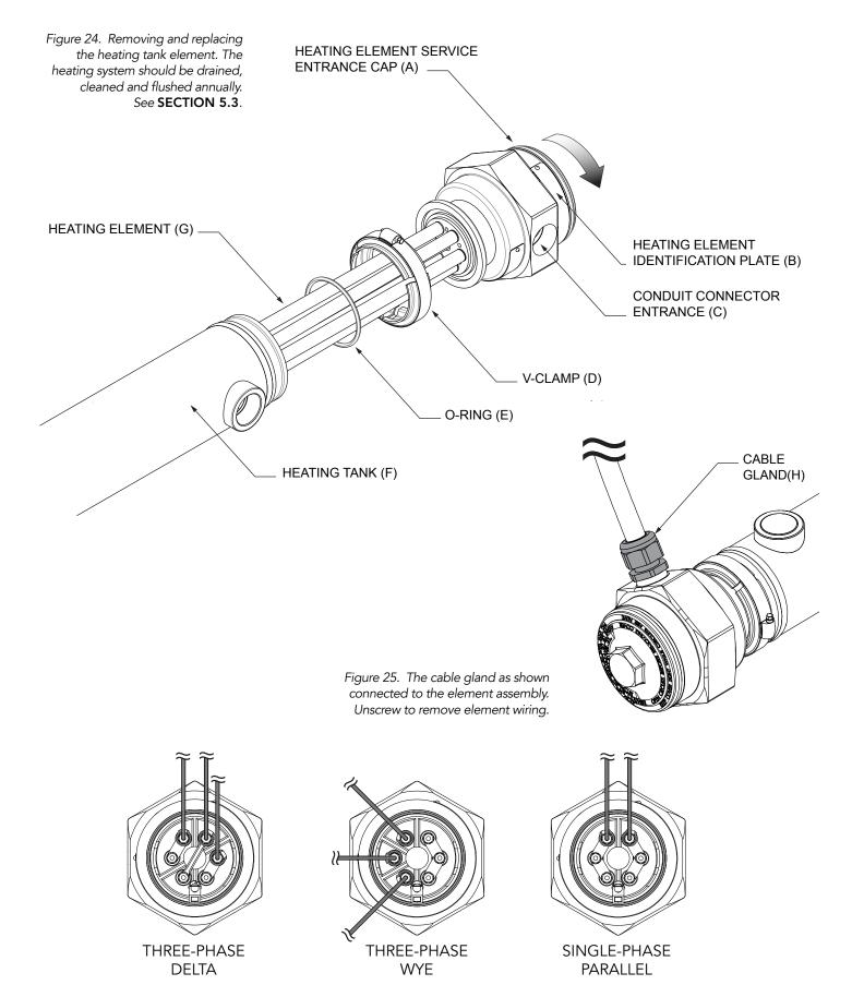
Figure 26. Heating tank element phase configurations. Replacement elements may be a different phase configuration.
