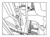
Figure 12. Typical oil discharge port (A) installed at locomotive engine lower P-pipe. Note coolant suction port (B) located at locomotive main engine drain.
