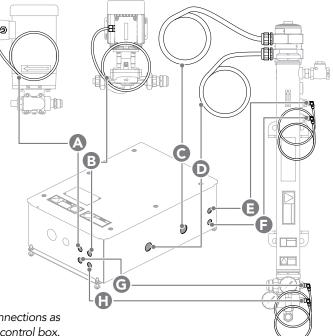
Figure 9. Pump, element and RTD connections as shown in the Modular DLV control box.
