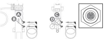
Figure 6. Tank assembly showing coolant high-limit RTD **(A)**, oil high-limit RTD **(B)**, coolant control RTD **(C)**, and oil control RTD **(D)**. Note RTD notch position (inset).
