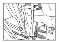
• To minimize flow restriction, the coolant supply line must be as short and as straight as possible. Use elbow fittings sparingly; HOTSTART recommends using sweeping bends or 45° fittings.
