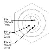
Figure 20. RTD pins 1, 3 and 4. The resistance between pin 1 and pin 3 should measure between 80 and 120 ohms. There should be continuity between pin 1 and pin 4.
