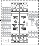
Figure 19. Control TCRs (TCR1, TCR3) showing terminals T1, T2 and T3.
