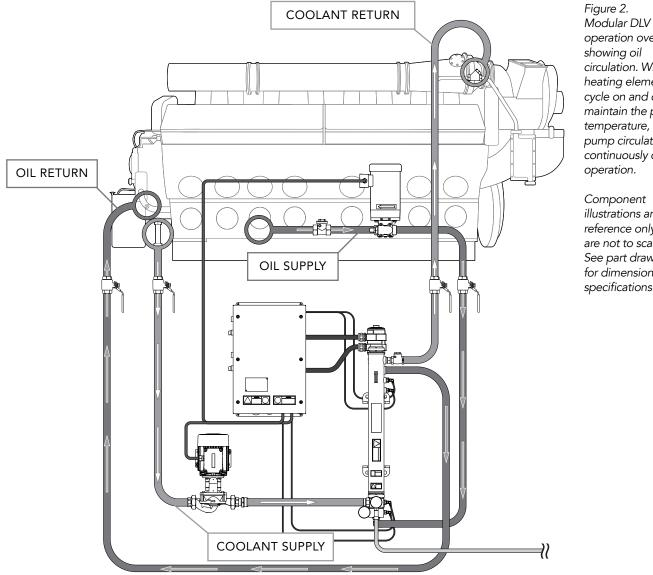
operation overview, showing oil circulation. While the heating elements cycle on and off to maintain the preset temperature, the pump circulates fluid continuously during operation.
