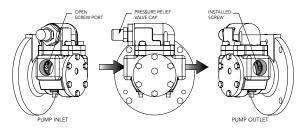
Figure 16. Modular DLV oil pump assembly. Note that the pressure relief valve cap must always point toward the inlet side of pump. Screw is installed on outlet side of pump.
