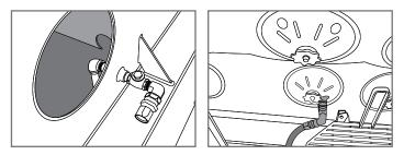
Figure 11. Typical oil suction port installations for railroad applications: near third inspection cover (left) and through cover (right).
