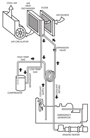
Heat is removed from the air and is transferred to the engine coolant system through pressurized refrigerant.
