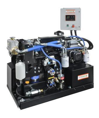
Hotstart's APU heating system is a self-contained coolant and oil preheater that uses the locomotive's onboard fuel supply to heat prime movers without requiring a shore power connection.
