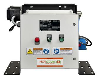
Hotstart's OSM heating system is an oil heater, developed to heat and circulate oil to maintain optimal temperatures for diesel and gas engines for stationary land power, marine and mining equipment.
