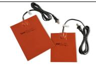
Hotstart Silicone Heating Pads are ideal for oil pans, engine blocks, hydraulic reservoirs, diesel fuel tanks and other fluid reservoirs. Constructed from a durable silicone/fiberglass material, these etched foil heating pads feature an easy peel-and-stick application. Silicone heating pads are for use on metal surfaces only.
