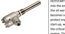
HOTSTART lube oil heaters thread into the engine's oil pan to keep the oil warm. When cold, oil becomes very viscous and may not protect engine components. Upon start-up, warm oil is supplied to the critical wear points in the engine. This reduces engine wear and allows easier starts which prolong battery life.
