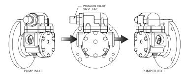
Figure 6. Typical OCLA pump assembly. Note that the pressure relief valve cap must always point toward the inlet side of pump.
