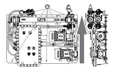
Figure 3. OCLA 0.438 inch (11.13 mm) diameter mounting holes × 6 (A). Mount unit in orientation shown. Do not mount at an angle or in any other orientation.
