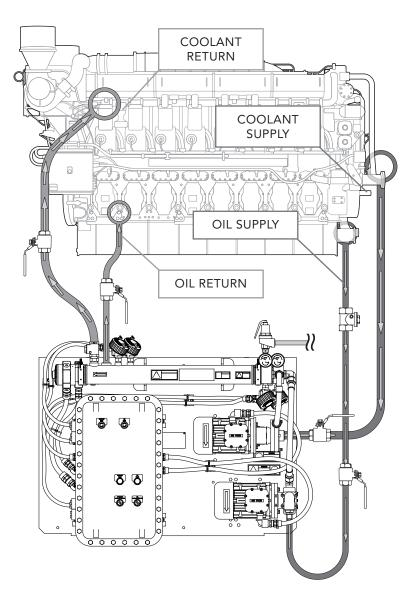
Figure 2. OCLA system operation. Component illustrations are for reference only and are not to scale. See part drawings for dimensions and specifications.
