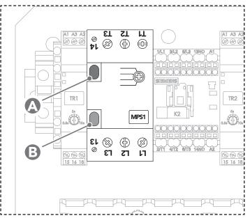
Figure 7. OCLA motor protection switch (left), showing stop/off (A) and reset/on (B) buttons. To reset the MPS, the heating system must be switched off and either the **RESET** button or the MPS reset/on button must be pressed.
