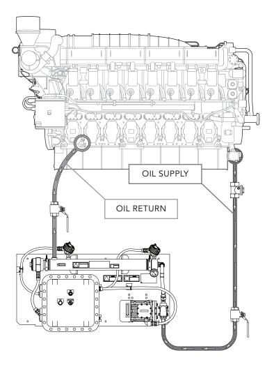
Figure 2. OLA system operation. Component illustrations are for reference only and are not to scale. See part drawings for dimensions and specifications.
