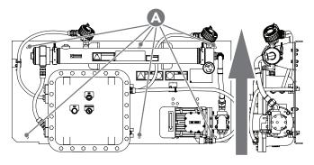
Figure 3. OLA 0.438 inch (11.13 mm) diameter mounting holes  $\times$  6 **(A)**. Mount unit in orientation shown. Do not mount at an angle or in any other orientation.
