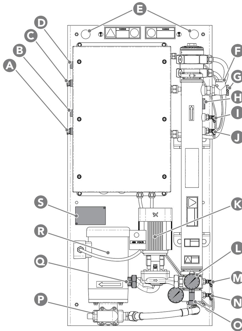
Figure 1. DLV heating system components.
