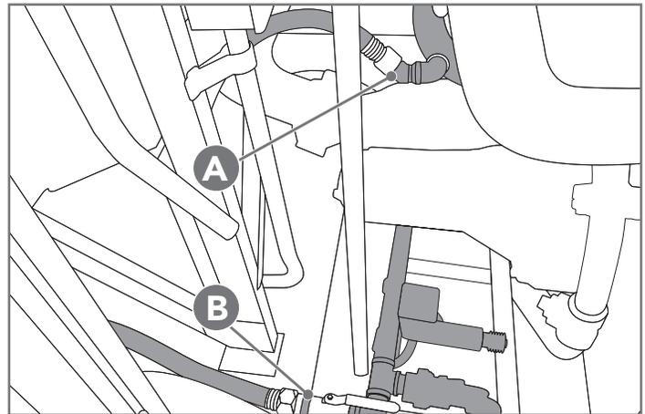
Figure 4. Typical oil discharge port (A) installed at locomotive engine lower P-pipe. Note coolant suction port (B) located at locomotive main engine drain.
