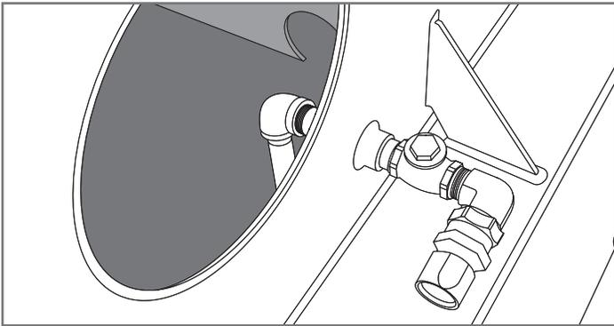
Figure 3. Typical oil suction port installations for railroad applications: near third inspection cover (above) and through cover (below).
