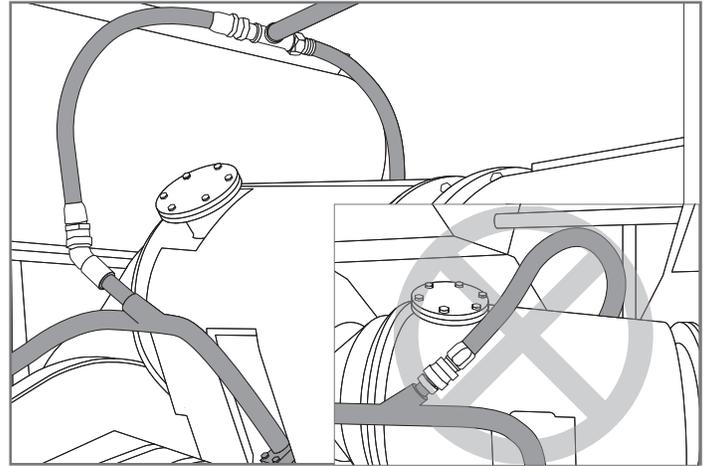
Figure 6. Typical coolant discharge ports installed on a turbocharged locomotive engine (above) and supercharged engine at Y-pipe (below). To distribute heat evenly, the return line is split into two discharge ports. Each port is installed at a welded 45° fitting, angled to ensure majority of heated coolant is transferred directly to engine block. Note incorrectly oriented fitting (inset). This fitting should be angled in the opposite direction to allow flow toward the engine.
