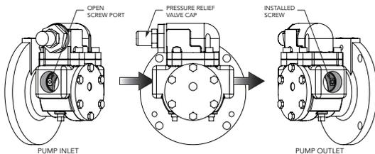
Figure 11. DLV oil pump assembly. Note that the pressure relief valve cap must always point toward the inlet side of pump. Screw is installed on outlet side of pump.
