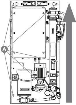
Figure 7. DLV 0.438 inch (11.13 mm) diameter mounting holes × 6 (A). Mount unit in orientation shown. Do not mount at an angle or in any other orientation.
