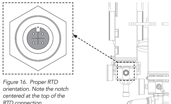
Figure 16. Proper RTD orientation. Note the notch centered at the top of the RTD connection.
