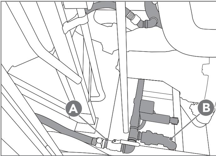
Figure 5. Coolant suction port installed at main locomotive engine drain. Note suction port (A) has been installed at the same level as the drain (B), ensuring DLV pump will draw water from the cooling system's lowest point.
