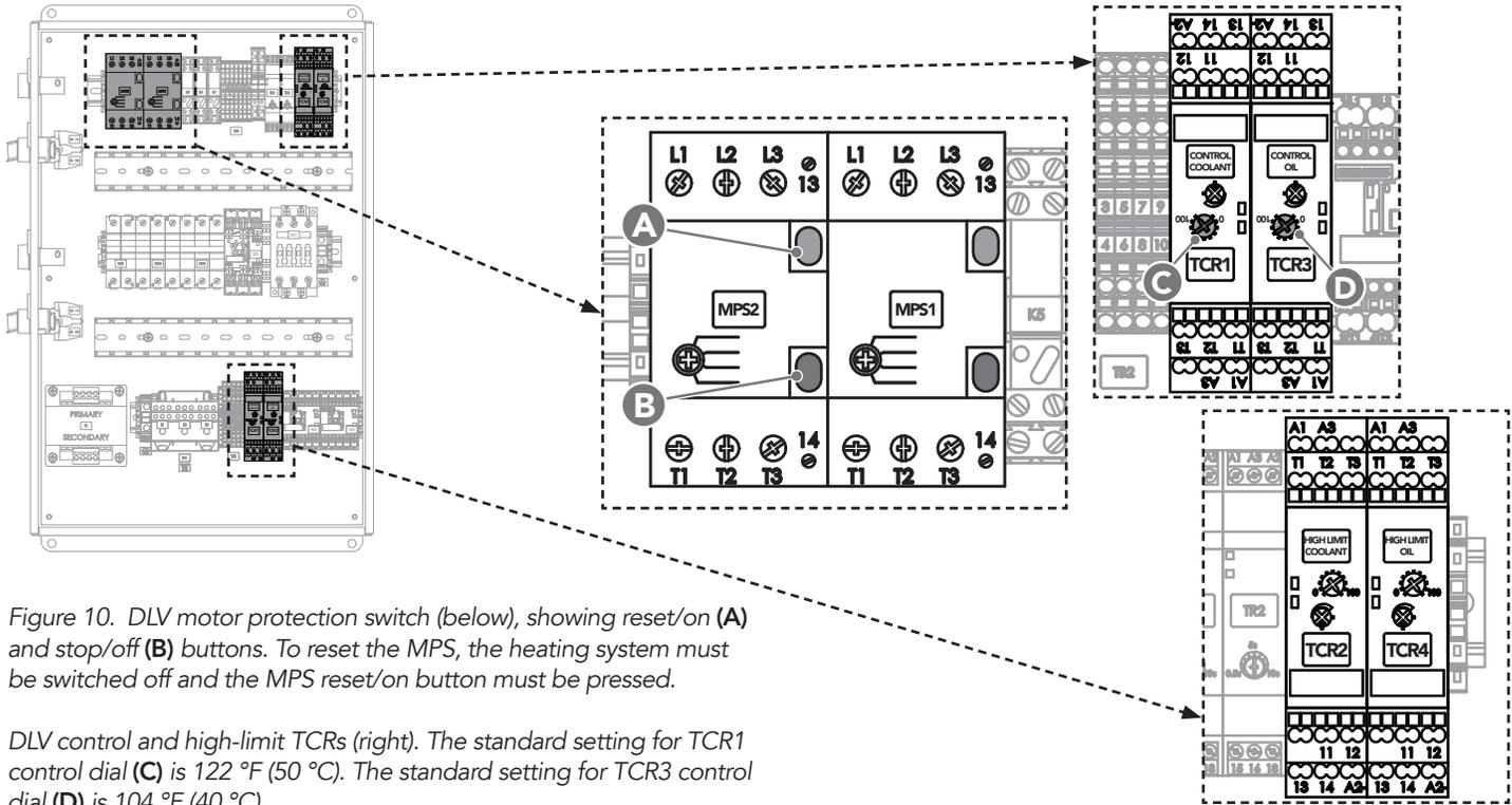
Figure 10. DLV motor protection switch (below), showing reset/on (A) and stop/off (B) buttons. To reset the MPS, the heating system must be switched off and the MPS reset/on button must be pressed.
