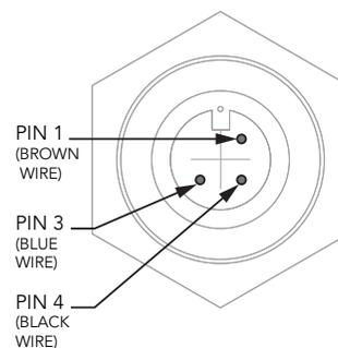
Figure 13. RTD pins 1, 3 and 4. The resistance between pin 1 and pin 3 should measure between 80 and 120 ohms. There should be continuity between pin 1 and pin 4.
