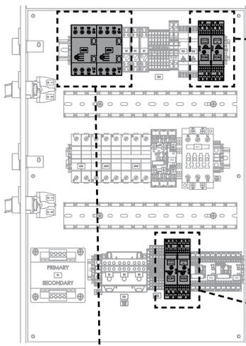
Figure 17. Modular DLV motor protection switch (below), showing reset/on (A) and stop/off (B) buttons. To reset the MPS, the heating system must be switched off and the MPS reset/on button must be pressed.
