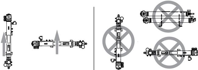
Figure 3. Correct heating tank assembly mounting orientations (left) and incorrect orientation (right). Incorrect positions show tank outlets positioned at bottom of tank or pointing downward.
