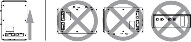
Figure 8. Correct control box orientation (left) and incorrect control box mounting orientations (right).
