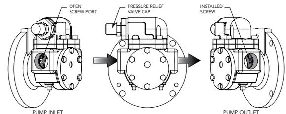
Figure 16. Modular DLV oil pump assembly. Note that the pressure relief valve cap must always point toward the inlet side of pump. Screw is installed on outlet side of pump.
