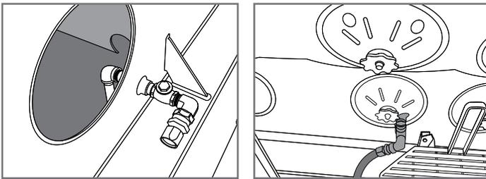
Figure 11. Typical oil suction port installations for railroad applications: near third inspection cover (left) and through cover (right).
