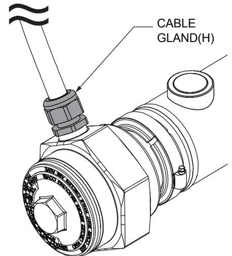
Figure 25. The cable gland as shown connected to the element assembly. Unscrew to remove element wiring.
