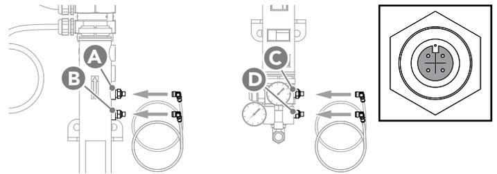
Figure 6. Tank assembly showing coolant high-limit RTD (A), oil high-limit RTD (B), coolant control RTD (C), and oil control RTD (D). Note RTD notch position (inset).
