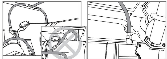
Figure 14. Typical coolant discharge ports installed on a turbocharged locomotive engine (left) and supercharged engine at Y-pipe (right). To distribute heat evenly, the return line is split into two discharge ports. Each port is installed at a welded 45° fitting, angled to ensure majority of heated coolant is transferred directly to engine block. Note incorrectly oriented fitting (inset). This fitting should be angled in the opposite direction to allow flow toward the engine.
