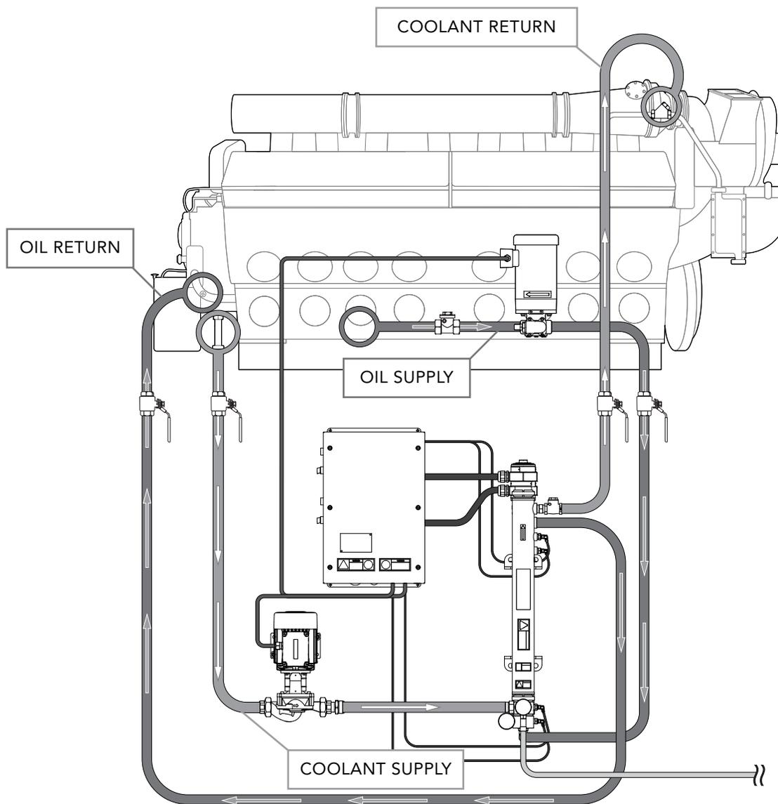
*Figure 2. Modular DLV operation overview, showing oil circulation. While the heating elements cycle on and off to maintain the preset temperature, the pump circulates fluid continuously during operation.*
