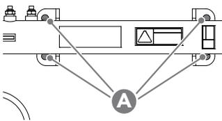
Figure 4. Modular DLV tank assembly .4 inch (10 mm) diameter mounting holes × 4 (A).
