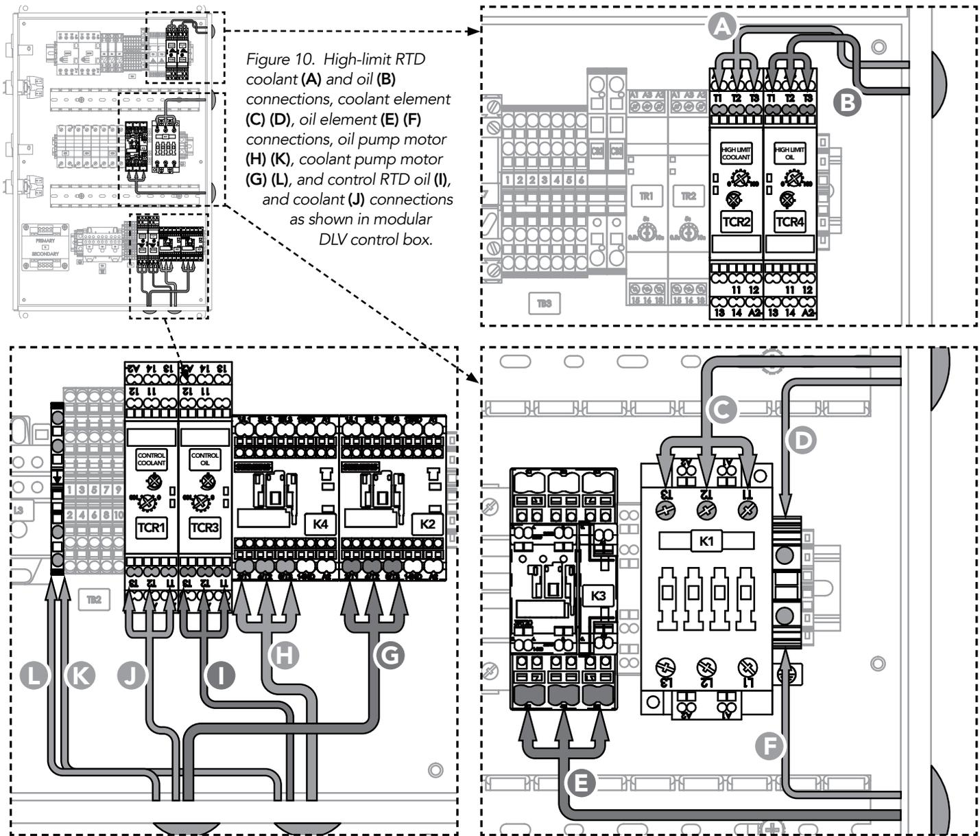
Figure 10. High-limit RTD coolant (A) and oil (B) connections, coolant element (C) (D), oil element (E) (F) connections, oil pump motor (G) (K), coolant pump motor (H) (L), and control RTD oil (I), and coolant (J) connections as shown in modular DLV control box.
