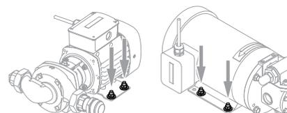
Figure 7. Coolant pump assembly and oil pump assembly showing .38 inch (10 mm) × 4 diameter mounting holes.
