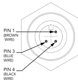
Figure 20. RTD pins 1, 3 and 4. The resistance between pin 1 and pin 3 should measure between 80 and 120 ohms. There should be continuity between pin 1 and pin 4.
