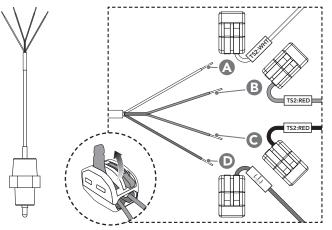
Figure 9. RTD leads and connectors shown on the RTD assembly, TSX:WHT (A), TSX:RED (red wire) (B), TSX:RED (black wire) (C), and Ground (D). Disconnect wire from connector as shown.
