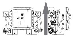
Figure 4. Mount unit in orientation shown. Do not mount at an angle or in any other orientation.
