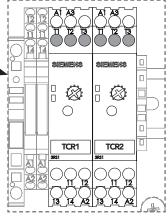
Figure 8. Control (TCR1) and high-limit (TCR2) TCR showing terminals T1, T2 and T3.
