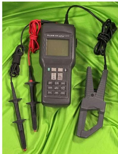
Figure 6: Fluke 41B Power Harmonics Analyzer
