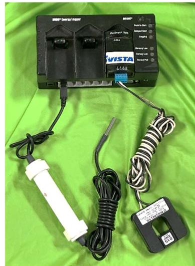
Figure 5: Onset H22 data logger, Onset TRMS module, a 15 amp current transducer (CT), and an Onset S-TMB-M002 temperature sensor.
