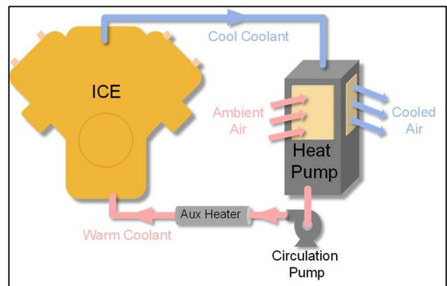
Figure 3: Generalized operational heating system diagram with heat pump, auxiliary (baseline) heater and heat pump controlled coolant circulation pump.
