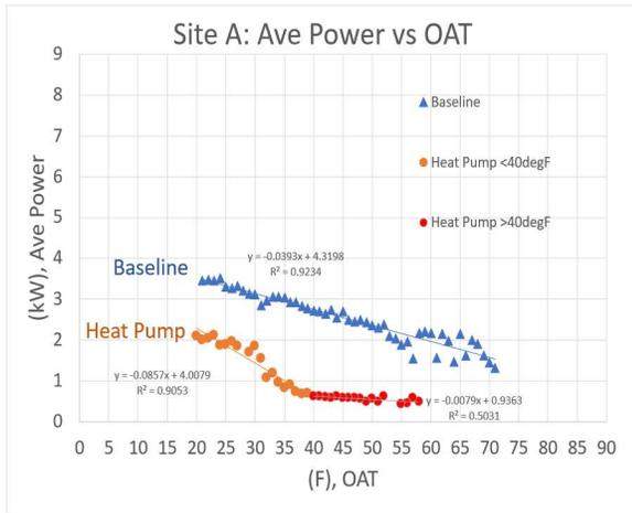
**Figure 7: Graph of binned average power consumption; note reporting period's two data sets above and below 40F.**
